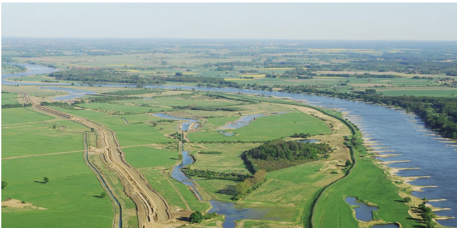
Natural water retention measures can offer cost effective solutions for the mitigation of flood risks and offer economically valuable benefits. Dike relocation near Lenzen, Germany. Photo: ©Jochen Purps
